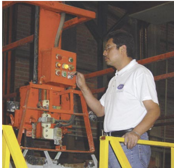
Most of the plating operations at Recubrimientos Metálicos de México are fully automated. Manuel Arenas, plating supervisor, is shown here with one of four hoists used for automatic zinc plating.
